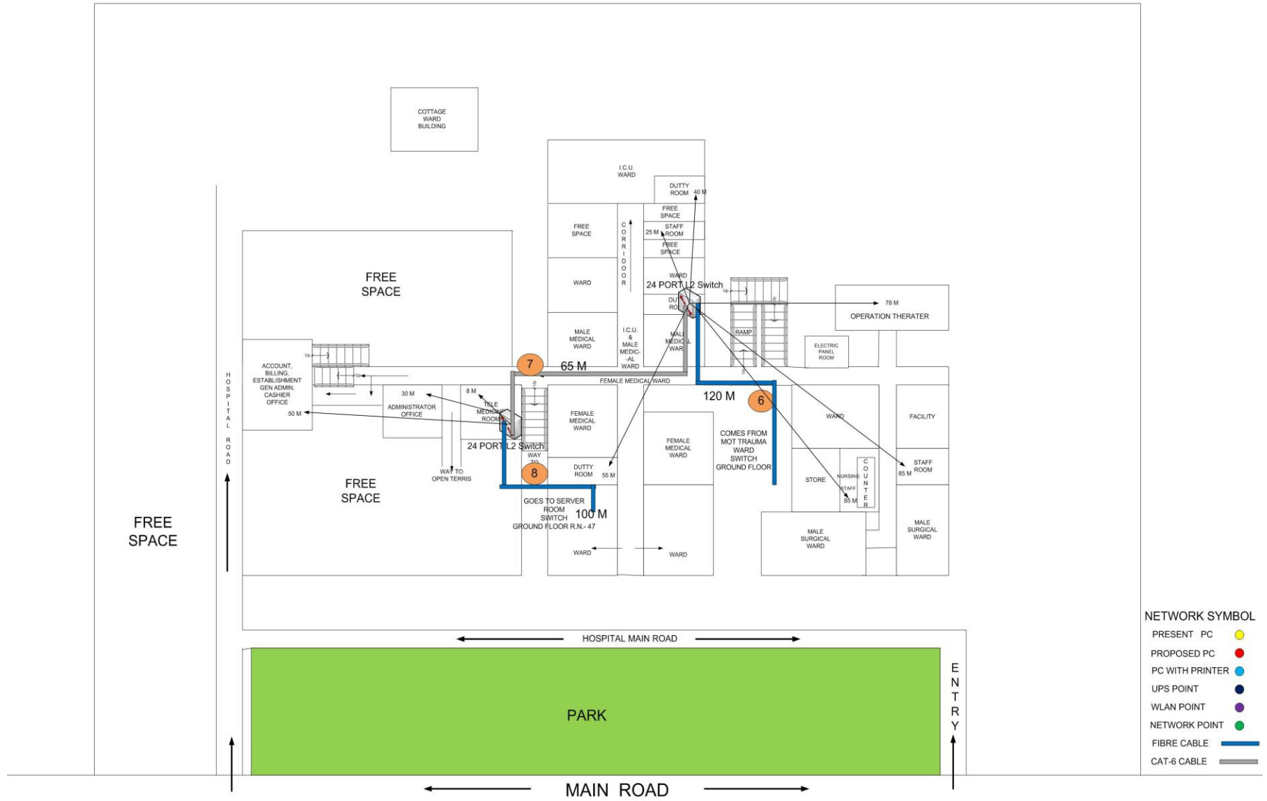
DH3.6 Dimensional Network Layout of First Floor of Shri Sanwaliya Ji General Building
